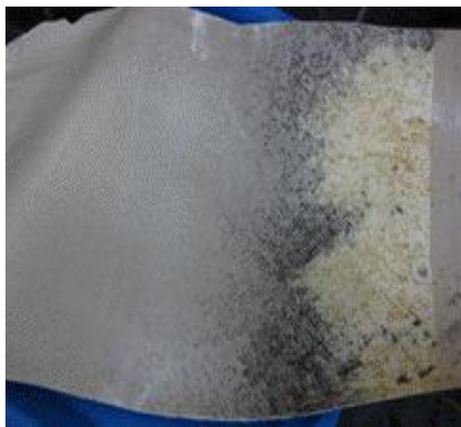
Figure 3.18 Scale delimiting a dry tubercle from a steel pipe surface.
