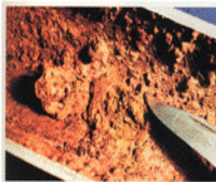
Figure 3.18 Scale delimiting a dry tubercle from a steel pipe surface.
