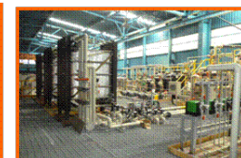
Recovery of wastewater from zinc-plating process for rinse water by EDR process ( China steel company, 700 m 3 /day)
